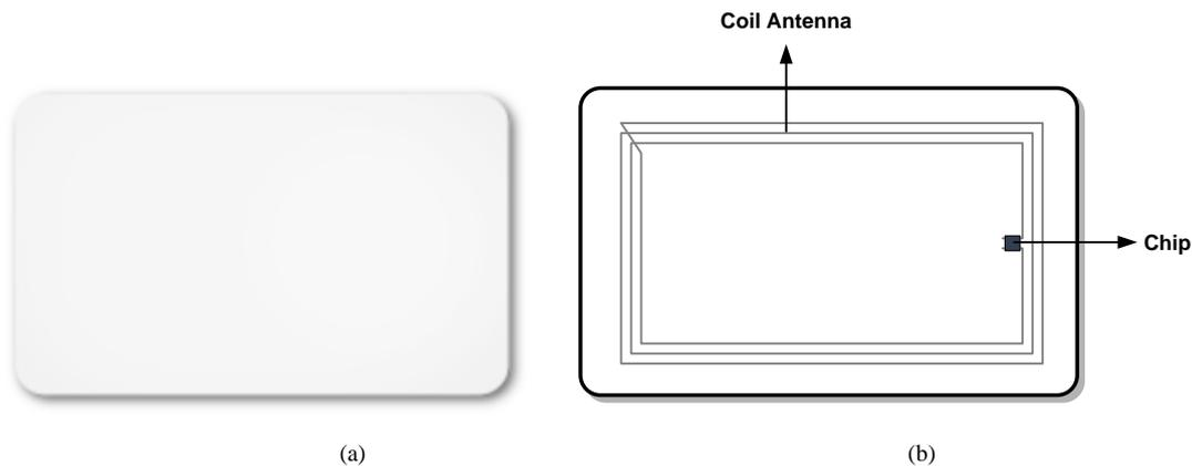
Figure 5. The RFID-card;
