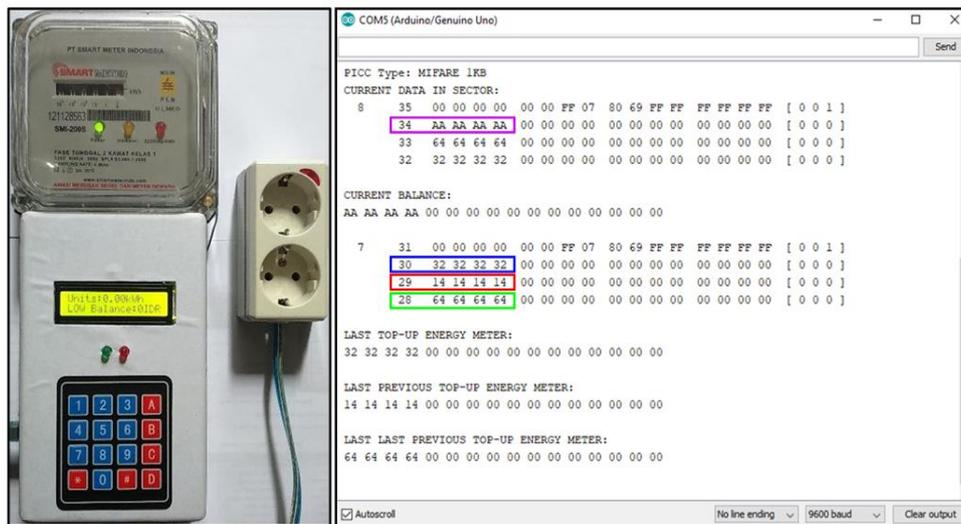
Figure 17. The conditions of the ETU and the RFID-card's memory before the credit top-up
