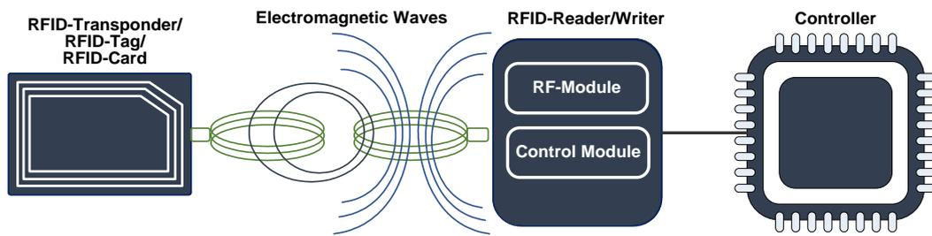
Figure 4. Basic components of an RFID system
