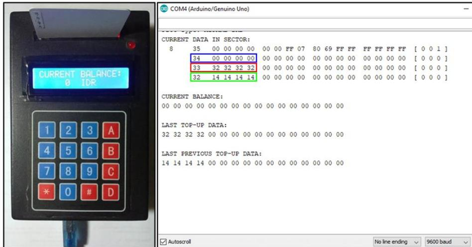
Figure 15. The conditions of the CTU and the RFID-card's memory before the balance top-up
