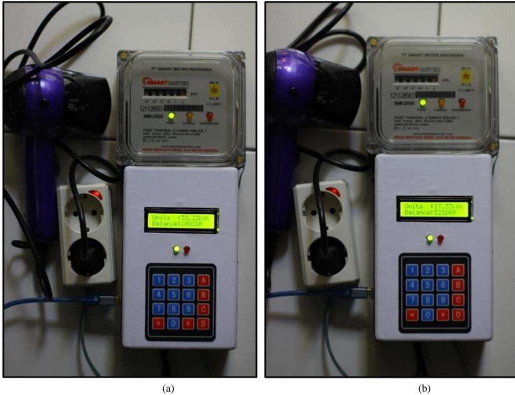
Figure 20. The operation of ETU and the energy credit deduction,
