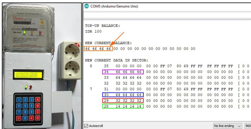
Figure 18. The conditions of the ETU and the RFID-card's memory after the credit top-up
