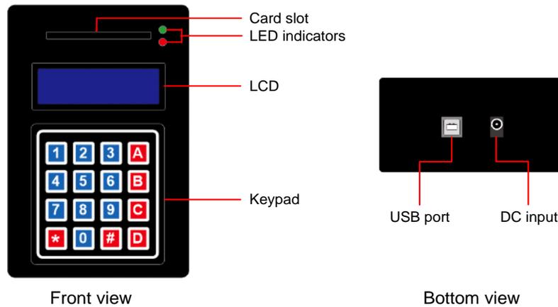
Figure 13. Design of CTU prototype
