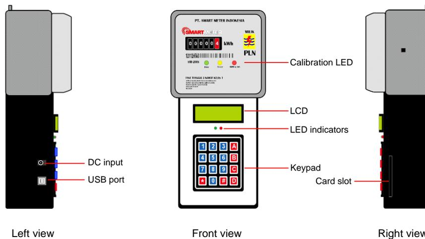
Figure 14. Design of ETU prototype
