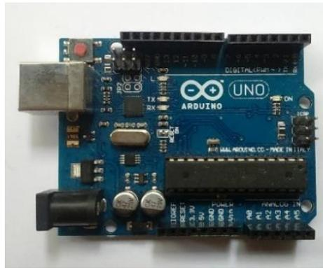
Figure 1. Arduino Uno board
