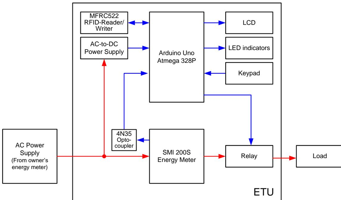
Figure 9. Block diagram of the ETU
