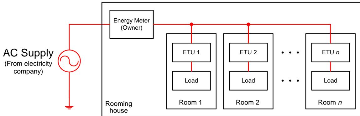
Figure 10. Implementation scheme of the proposed system
