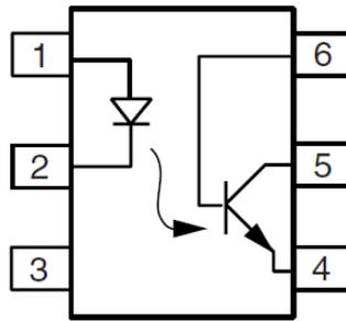
Figure 7. 4N35 Optocoupler and its pinout [22]
