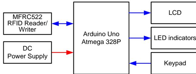
Figure 8. Block diagram of the CTU
