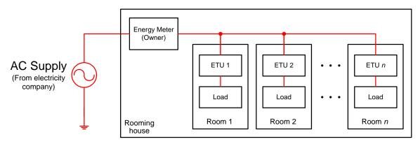
Figure 10. Implementation scheme of the proposed system
