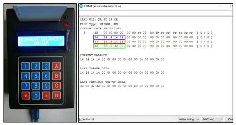
Figure 16. The conditions of the CTU and the RFID-card's memory after the balance top-up
