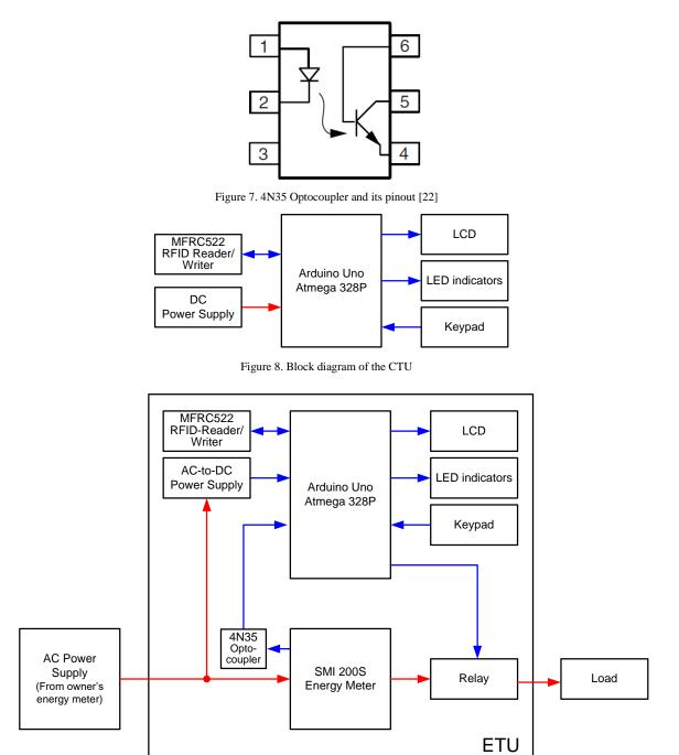
Figure 9. Block diagram of the ETU
