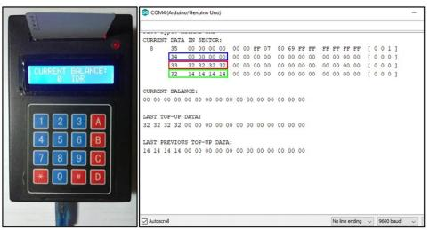
Figure 15. The conditions of the CTU and the RFID-card's memory before the balance top-up
