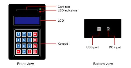
Figure 13. Design of CTU prototype
