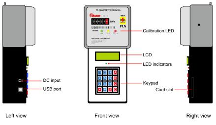
Figure 14. Design of ETU prototype
