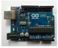
Figure 1. Arduino Uno board
