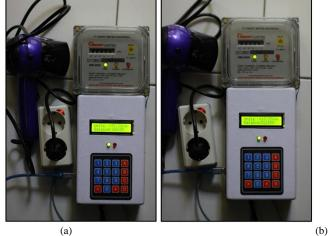
Figure 19. The operation of ETU and the energy credit deduction, (a) Initial condition; (b) Final condition
