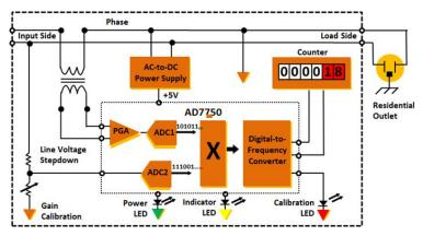
Figure 2. Functional block diagram of a single-phase power meter using AD7750 [15].
