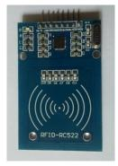
Figure 6. RFID MFRC522
