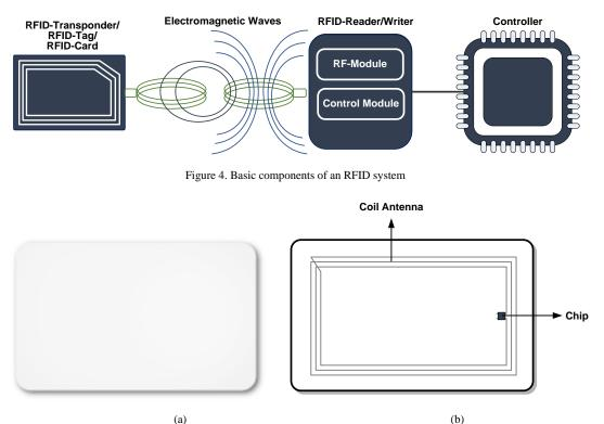
(a) Figure 5. The RFID-card; (a) The blank card; (b) The transponder inlays within the card
