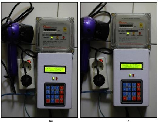
(a)Figure 20. The operation of ETU and the energy credit deduction,(a) Initial condition; (b) Final condition
