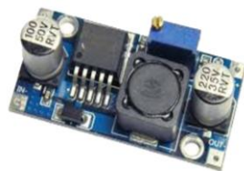
Figure 4. Step-Up Buck-Boost Converter
